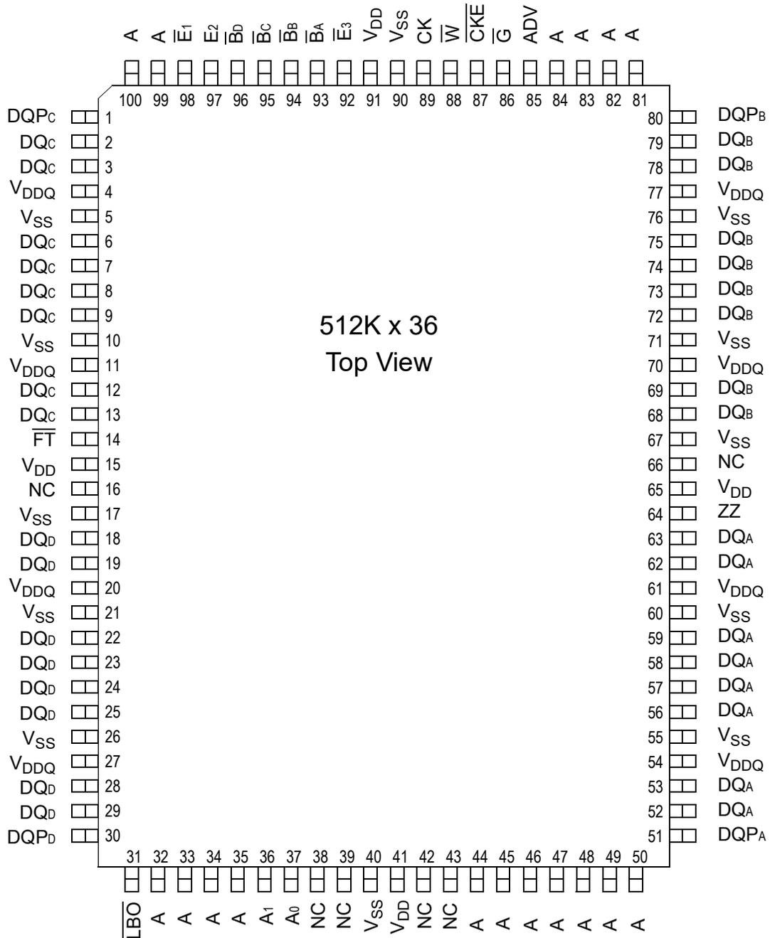
**100-Pin TQFP Pin Descriptions**
