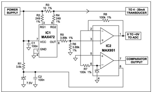
Figure 1. This circuit derives a 0V-5V output from a 4-20mA current-loop signal, using a load resistor of only  $10\Omega$ .
