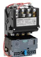
Non-reversing motor starter Size 0 Three phase full voltage Solid-state overload relay OLRelay amp range 3-12A 110VAC 50HZ / 120VAC 60HZ coil Combination type No enclosure
