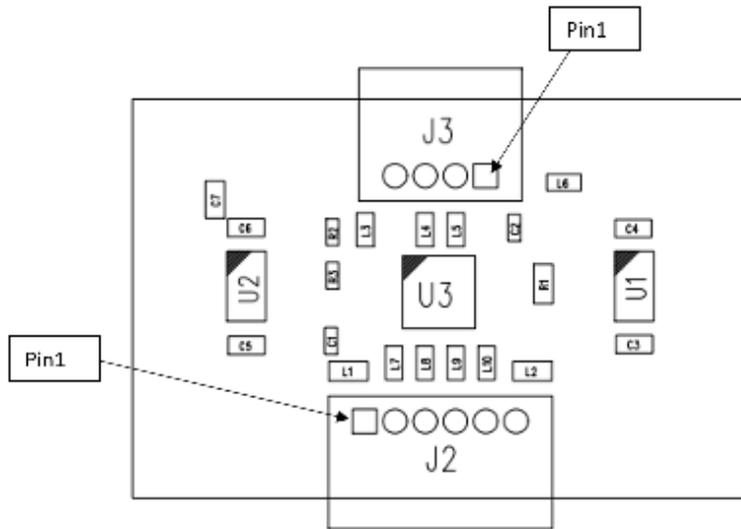
**FIGURE 4: TOP VIEW OF RS-422 ADAPTER WITH PIN 1 CALLED OUT FOR EACH CONNECTOR**
