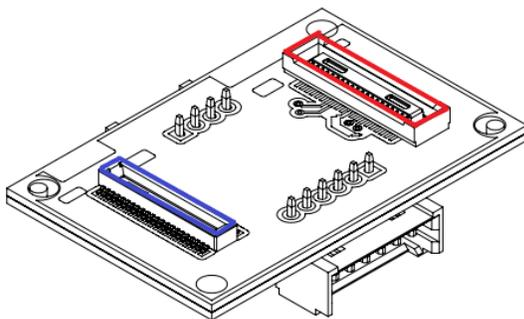
FIGURE 2: RS-422 ADAPTER WITH MALE/FEMALE CONNECTORS CALLED OUT
