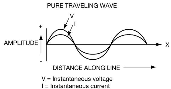
Pure traveling waves: V & I in the lossless case are in phase. V & I also reverse polarity every half wavelength.
