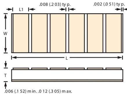
GA SERIES MULTIPLE PAD SLCs are ideal for circuits such as MMIC devices requiring multiple capacitance applications, i.e., bypassing and bias circuits. The GA Multicaps in the Selection Guide below are listed using KAVX's GA and K dielectrics, with a pad length of .015 (.380). However, other array designs are possible. Please consult factory.
