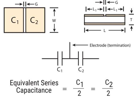
Terminations C1 and C2 may be mounted directly to the microstrip line or with the top electrode (termination) facing down in the flip chip configuration.
