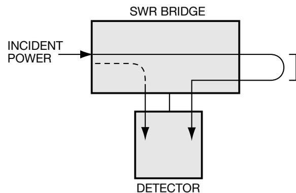
Figure 5. Return Loss Measurement: Establishing a Reference
