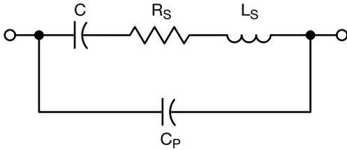
Figure 8. Equivalent Circuit of a Microwave Capacitor
