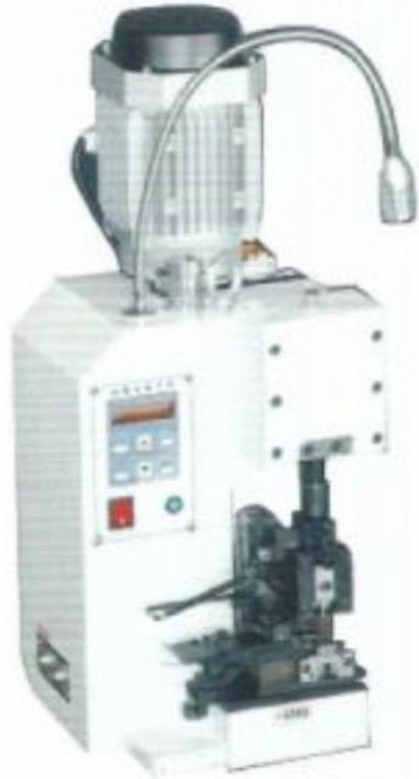
SEMI-AUTOMATED CRIMP MACHINE SHOWN WITH APPLICATOR
