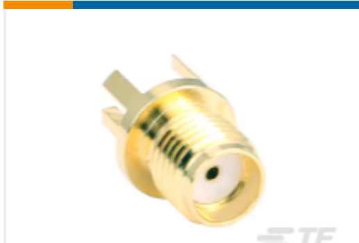
TE Part # L9000267-01 SMA Jack 50 Ohm .062 PCB Edge Mount gold
