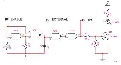
Figure 9. Transmitter board schematic.
