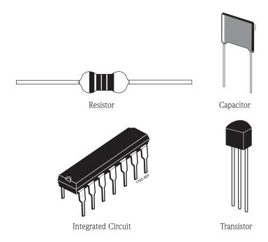
Figure 1. Component identification: resistors, capacitors, ICs.
