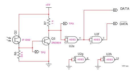
Figure 10. Circuit diagram of receiver.
