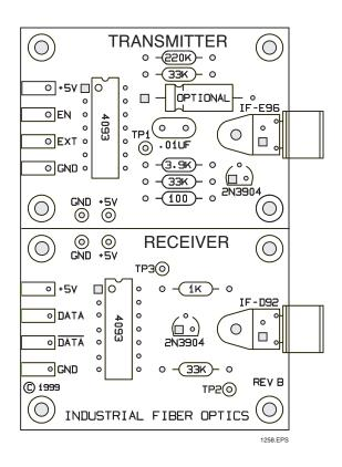
Figure 2. Board details on the printed wiring boards.
