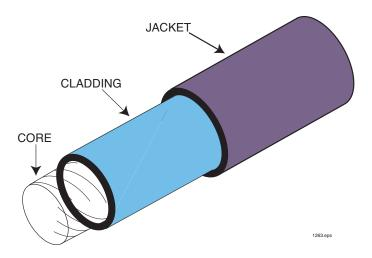
Figure 8. Cross-section of a simple fiber optic cable.
