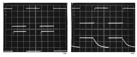
Figure 5. Two oscilloscope traces of: a) transmitter TP1 (top) and receiver TP3 (bottom) signals; and b) receiver TP3 (top) and TP2 (bottom) signals.
