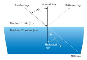
Figure 6. Different portions of a light ray at a material interrace.
