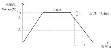
容量计算公式 Capacitance calculation formula:  $C = \frac{I \times (t_2 - t_1)}{U_1 - U_2}$
