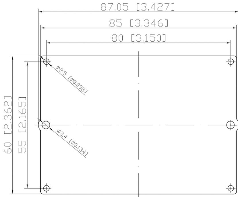
Pic. 2. qGround AFC PCB Kit PCB dimensions
