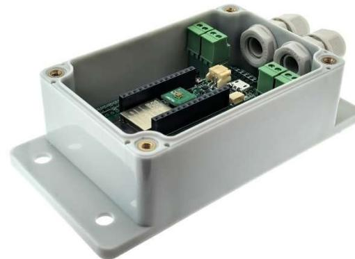
Pic. 15. qBoard light sensor controller
