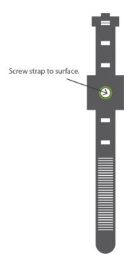
2) Wrap strap around S2C Link and tighten strap to secure the product.
