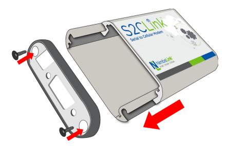
3.1.5 Step 5: Insert the PCB assembly into the enclosure. The side of the PCB with the DB9 should be inserted first. Make sure it is not inserted upside down. Be sure to copy the MEID/IMEI/SIM ID from the Skywire so it is easily accessible after the device has been assembled.
