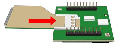
**3.1.2** Step 2: Insert the Skywire into the base board. The antenna ports on the Skywire should be facing the SMA ports on the base board.
