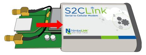
**3.1.6** Step 6: Attach the RF face plate to the enclosure. Make sure that the SIM extender is aligned to the slot in the middle of the face plate for the SIM card.
