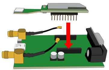
**3.1.3** Step 3: Attach the U.FL connectors to the Skywire. To prevent damaging the U.FL connectors a U.FL extractor tool should be used.
