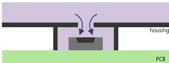
Figure 3. A large opening in the housing provides improved air exchange and thus enhanced access to the environment.
