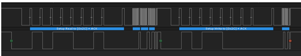
Figure 9: I3C data package
