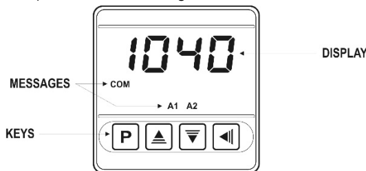
Figure 6 – Identification of the front panel parts
