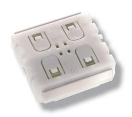
PTM 216Z pushbutton transmitter modules are self-powered (no batteries) and fully maintenance-free. They can therefore be used in all environments including locations that are difficult to reach or within hermetically sealed housings.
