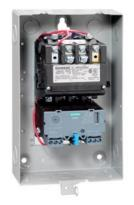
Non-reversing motor starter Size 1 Three phase full voltage Solid-state overload relay OLRelay amp range 0.25-1A 240VAC 50HZ / 277VAC 60HZ coil Combination type Indoor general purpose use
