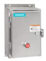
Non-reversing motor starter Size 1 Three phase full voltage Solid-state overload relay OLRelay amp range 0.75-3.4A 190-220/220-240V 50/60HZ coil Combination type Water/dust tight non-corrosive
