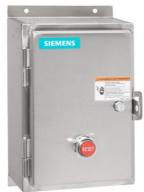
Non-reversing motor starter Size 1 Three phase full voltage Solid-state overload relay OLRelay amp range 3-12A 208VAC 60HZ coil Combination type Water/dust tight non-corrosive
