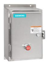
Non-reversing motor starter Size 3 1/2 Three phase full voltage Solid-state overload relay OLRelay amp range 50-200A 220-240/440-480VAC 60HZ coil Combination type Water/dust tight non-corrosive
