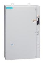
Non-reversing motor starter, Size 2 1/2, Three phase full voltage, Solid-state overload relay, OLRelay amp range 25-100A, 380 440/440 480V 50/60HZ coil, Combination type, 100A non-fusible disconnect, Enclosure NEMA type 4/12, Water/dust tight for outdoors, Standard width enclosure
