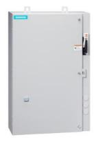
Non-reversing motor starter Size 4 Three phase full voltage Solid-state overload relay OLRelay amp range 50-200A 380-440/440-480V 50/60HZ coil Combination type 150A circuit breaker Enclosure NEMA type 4/12 Water/dust tight for outdoors Standard width enclosure
