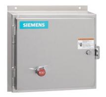
Reversing motor starter, Size 1, Three phase full voltage, Solid-state overload relay, OLR amp range 10-40A, Non-combination type, Encl. type 4X 304 S. Steel, Water/dust tight noncorrosive, Standard width enclosure
