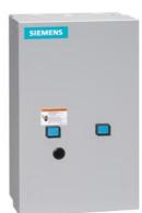
2-speed 3-phase motor starter Size 0 Two separate windings Constant or variable torque Solid-state overload relays Low SPD OLR range 0.75-3.4A High SPD OLR range 0.75-3.4A 110V 50HZ / 120V 60HZ coil Enclosure NEMA type 1 Indoor general purpose use
