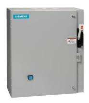
2-Speed 3-phase motor starter Size 1 Two separate windings Constant or variable torque Solid-state overload relays Low SPD OLR range 3-12A High SPD OLR range 5.5-22A 110V 50HZ / 120V 60HZ coil Combination type 30Amp disconnect switch Enclosure NEMA type 4/12 Water/dust tight for outdoors
