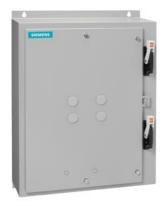
Duplex starter w/o alternator Size 1 Three phase full voltage Solid-state overload relay OLR amp range 5.5-22A 208VAC 60Hz Coil Combination type Two 30A disconnect switches Encl NEMA type 4 painted steel Water/dust tight weather proof
