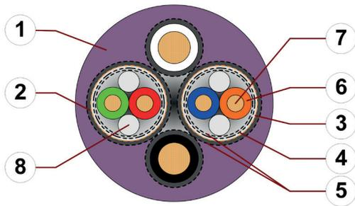
1. Outer jacket: Pressure extruded, gusset-filling, flame-retardant TPE mixture
