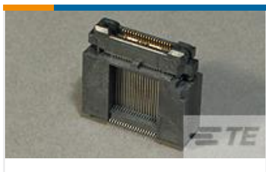
TE Part # 5767017-1 MICT,900PLUG,38,ASSY,.025,REC
