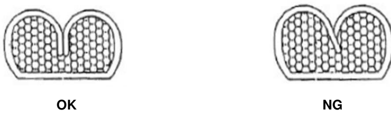
Fig.5 Conductor Crimping Image in cross section (In case of flat bottom shape)
