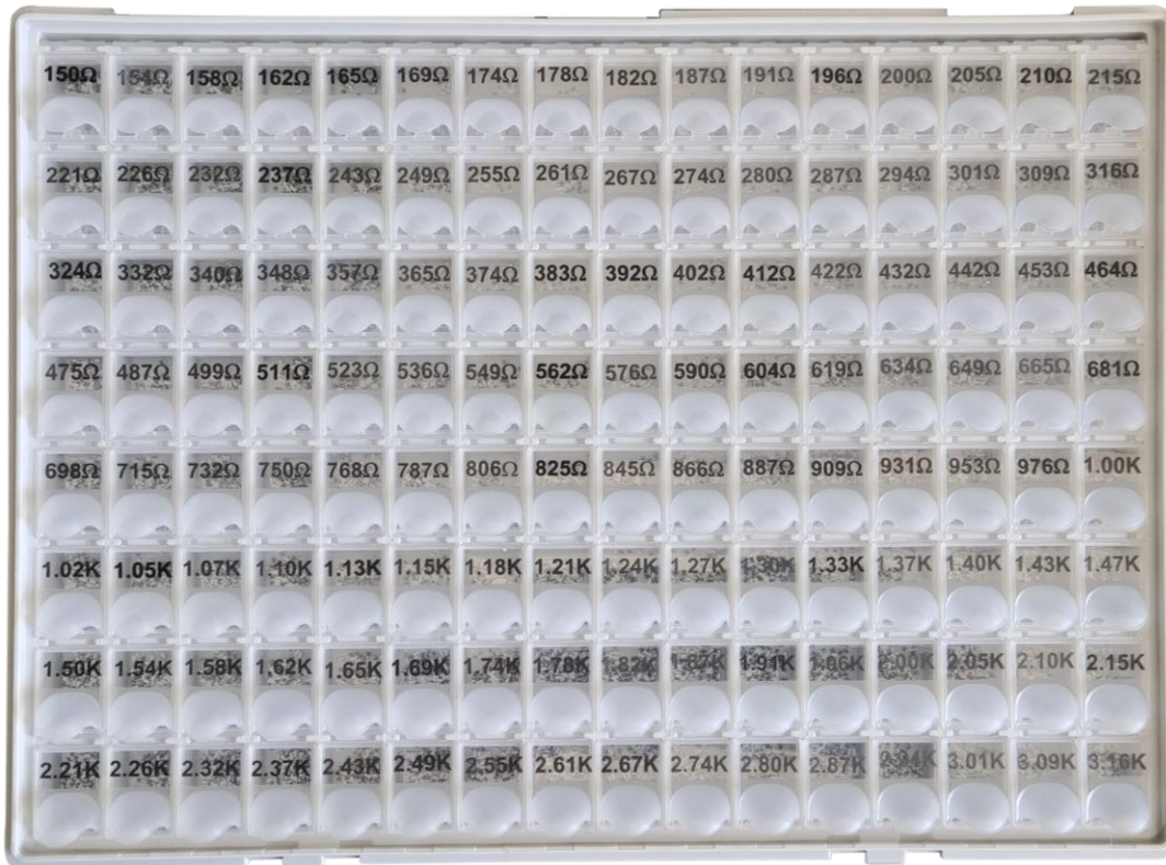
Figure 7. 510 Value Resistor Kit 4-2 Bin Layout
