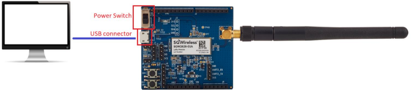
Figure 2: SGW2828-EVK to PC Connection
