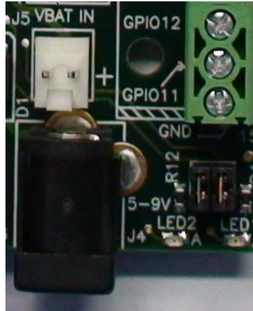
Figure 5 - LEDs enabled (both jumpers installed)
