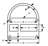
METALASTIC GASKET TOLERANCES inches (mm) DIMENSIONS TOLERANCES A All Die-cut Dimensions ±0.015 (±0.38) 0.140 (3.56) Expanded Foil B Min. Width Woven Wire 0.125 (3.18) Expanded Foil 0.090 (2.28) C Min. Wall Thickness Woven Wire 0.080 (2.03) If min. wall thickness C cannot be D Slot accommodated, holes should be changed to slots.
