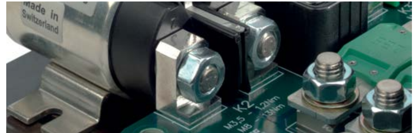
Attaching a high-current relay onto an angled PowerElement
