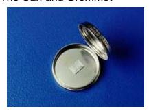
An iButton device uses its stainless steel 'can' as an electronic communications interface. Each can has a data contact, called the 'lid', and a ground contact, called the 'base'. Each of these contacts is connected to the silicon chip inside. The lid is the top of the can; the base forms the sides and the bottom of the can and includes a flange to simplify attaching the button to just about anything. The two contacts are separated by a polypropylene grommet.
