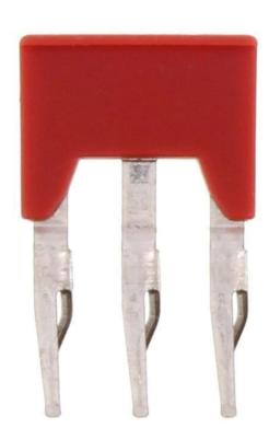
Insulated cross-connector, No. of poles: 3, Mounting type: Plug in, Width: 16.2 mm, Rated cross-section: 4 mm², Colour: Red
