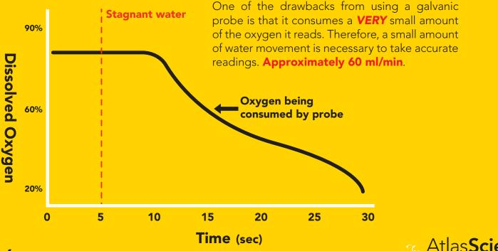
This galvanic dissolved oxygen probe is a passive device that generates a small voltage from 0mv - 60+mv depending on the oxygen saturation of the sensing membrane. This voltage can easily be read by a multimeter or an analog to digital converter.
