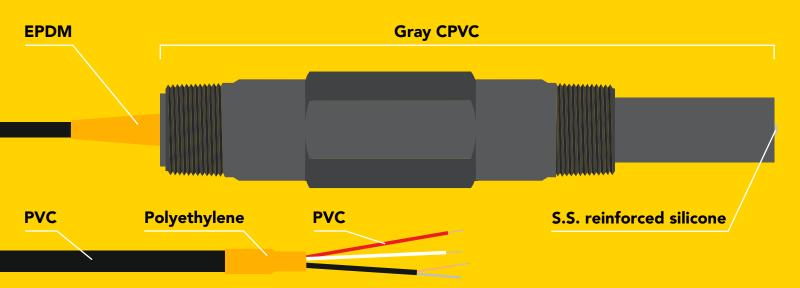
This Dissolved Oxygen probe can be fully submerged in fresh or salt water, up to the Tinned leads indefinitely.
