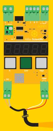
For industrial purposes, the Industrial Dissolved Oxygen probe connects easily to our *Industrial D.O. Transmitter.*
