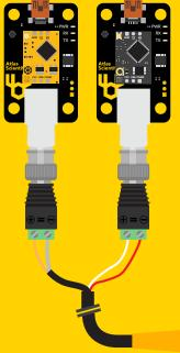
Using two **BNC with Terminal Screws**, you can easily connect the Industrial Dissolved Oxygen probe to our **EZO<sup>TM</sup> D.O. Circuit** and **EZO<sup>TM</sup> RTD Circuit** via our **Electrically Isolated USB EZO<sup>TM</sup> Carrier Board.**
